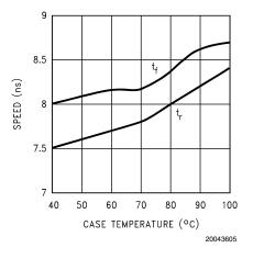
FIGURE 4. Speed vs Temp.
