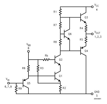
FIGURE 1. Simplified Schematic Diagram (One Channel)
