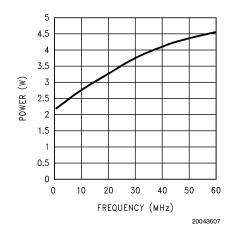
FIGURE 6. Power Dissipation vs Frequency
