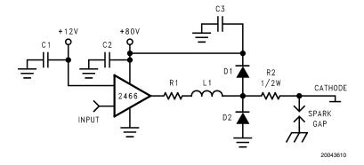
FIGURE 9. One Channel of the LM2466 with the Recommended Application Circuit
