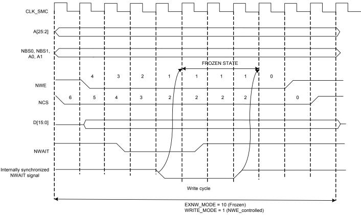
Figure 27-27. Write Access with NWAIT Assertion in Frozen Mode (EXNW\_MODE = 10).
