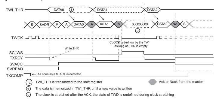
Figure 24-26. Clock Synchronization in Read Mode
