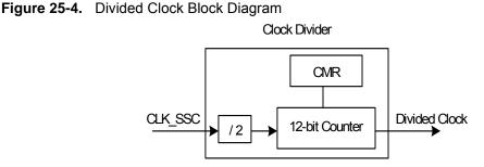
The Master Clock divider is determined by the 12-bit field DIV counter and comparator (so its maximal value is 4095) in the Clock Mode Register CMR, allowing a Master Clock division by up to 8190. The Divided Clock is provided to both the Receiver and Transmitter. When this field is programmed to 0, the Clock Divider is not used and remains inactive.
