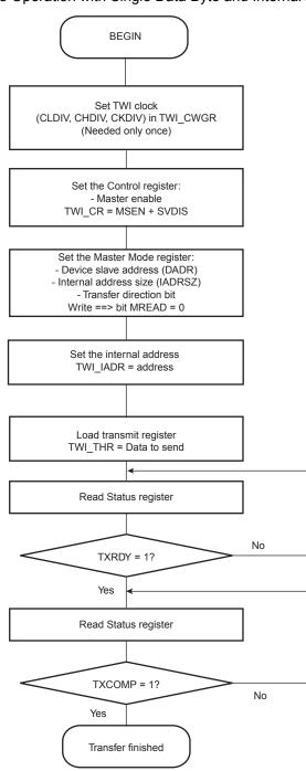
Figure 24-14. TWI Write Operation with Single Data Byte and Internal Address
