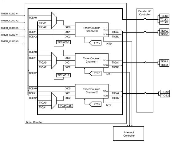
Figure 31-1. Timer Counter Block Diagram
