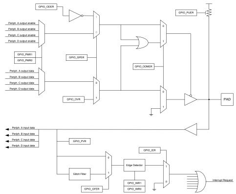
Figure 22-1. Overview of the GPIO pad connections
