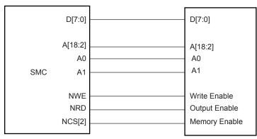
Figure 27-4. Memory Connection for an 8-bit Data Bus
