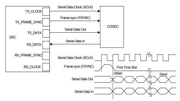
Figure 25-19. Time Slot Application Block Diagram
