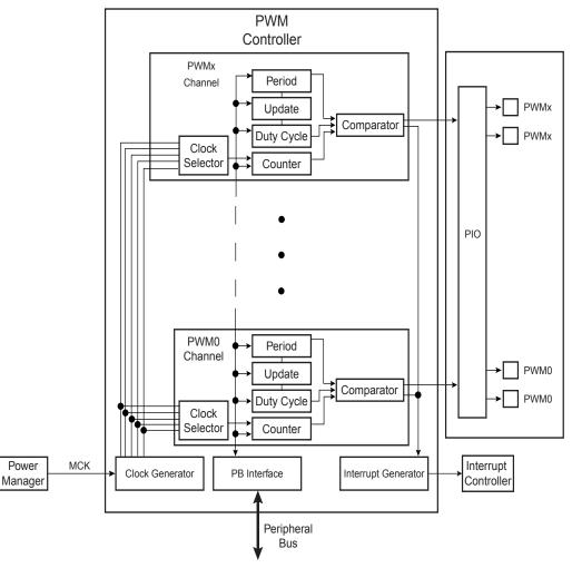
Figure 32-1. Pulse Width Modulation Controller Block Diagram
