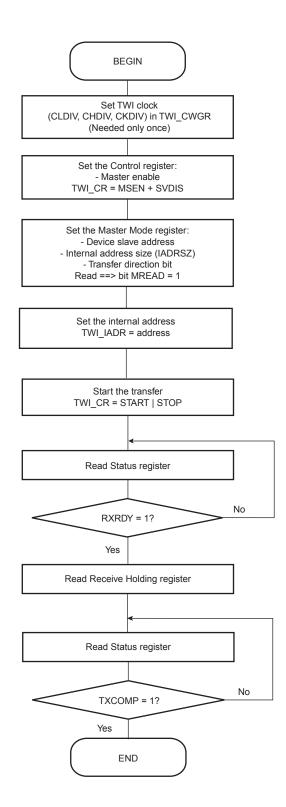
Figure 24-17. TWI Read Operation with Single Data Byte and Internal Address
