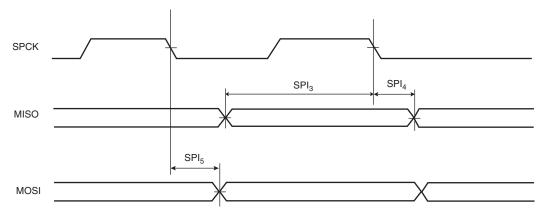
Figure 38-7. SPI Master mode with (CPOL=0 and NCPHA=1) or (CPOL=1 and NCPHA=0)
