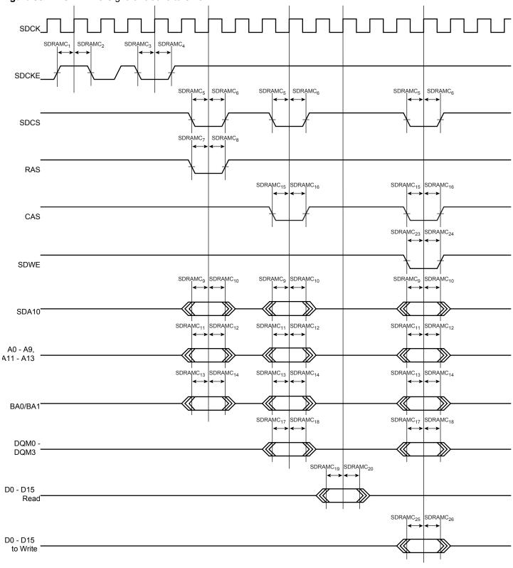
Figure 38-4. SDRAMC Signals relative to SDCK.
