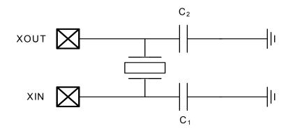
Figure 13-2. Oscillator connections
