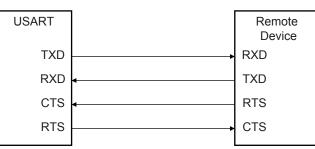
Figure 26-27. Connection with a Remote Device for Hardware Handshaking
