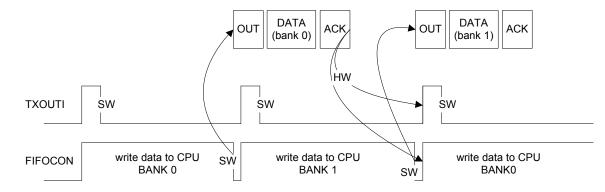
Figure 30-29. Example of an OUT Pipe with 2 Data Banks and a Bank Switching Delay
