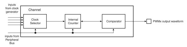
Each of the 7 channels is composed of three blocks:
