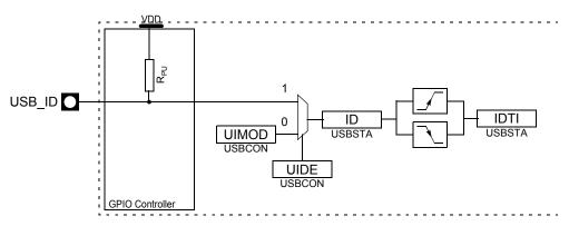
The USB mode (device or host) can be either detected from the USB\_ID pin or software selected from the UIMOD bit, according to the UIDE bit. This allows the USB\_ID pin to be used as a general purpose I/O pin even when the USB interface is enabled.
