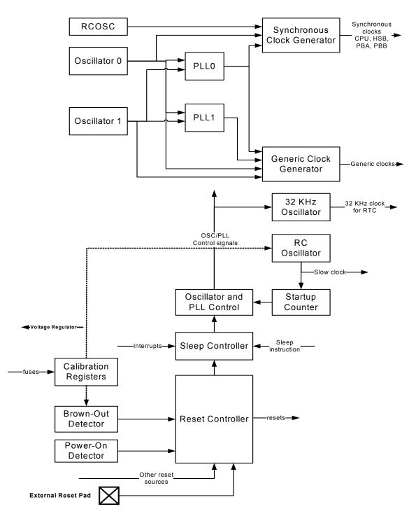
Figure 13-1. Power Manager block diagram
