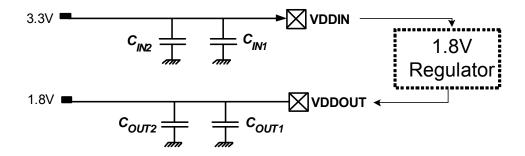
Refer to Section 38.3 on page 765 for decoupling capacitors values and regulator characteristics
