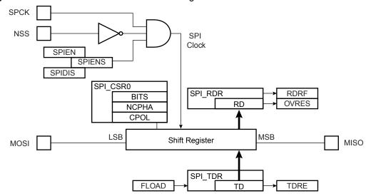
Figure 23-9. Slave Mode Functional Block Diagram
