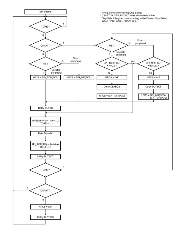
Figure 23-6. Master Mode Flow Diagram S
