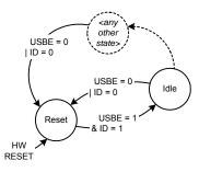
After a hardware reset, the USB controller device mode is in the Reset state. In this state:
