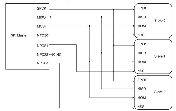
Figure 23-2. Application Block Diagram: Single Master/Multiple Slave Implementation
