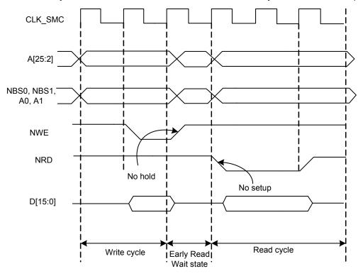
Figure 27-18. Early Read Wait State: Write with No Hold Followed by Read with No Setup.
