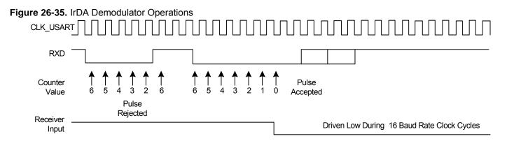
As the IrDA mode uses the same logic as the ISO7816, note that the FI\_DI\_RATIO field in FIDI must be set to a value higher than 0 in order to assure IrDA communications operate correctly.
