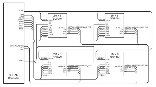
Figure 28-3. SDRAM Controller Connections to SDRAM Devices: 16-bit Data Bus Width
