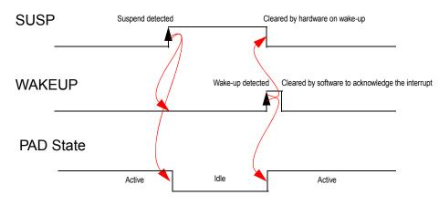
The Suspend interrupt flag (SUSP) is set and the Wake-Up interrupt flag (WAKEUP) is cleared when a USB "Suspend" state has been detected on the USB bus. This event automatically puts the USB pad in the Idle state. The detection of a non-idle event sets WAKEUP, clears SUSP and wakes up the USB pad.
