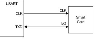
When operating in ISO7816, either in T = 0 or T = 1 modes, the character format is fixed. The configuration is 8 data bits, even parity and 1 or 2 stop bits, regardless of the values programmed in the CHRL, MODE9, PAR and CHMODE fields. MSBF can be used to transmit LSB or MSB first. Parity Bit (PAR) can be used to transmit in normal or inverse mode. Refer to "USART Mode Register" on page 343 and "PAR: Parity Type" on page 345.
