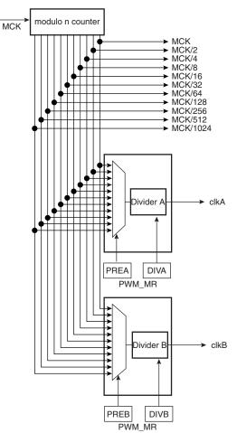
**Caution:** Before using the PWM macrocell, the programmer must ensure that the PWM clock in the Power Manager is enabled.
