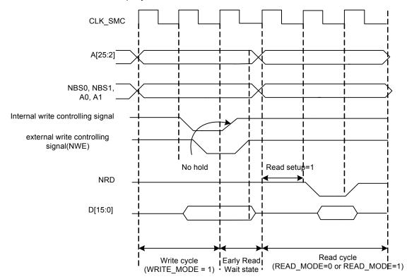
Figure 27-20. Early Read Wait State: NWE-controlled Write with No Hold Followed by a Read with one Set-up Cycle.
