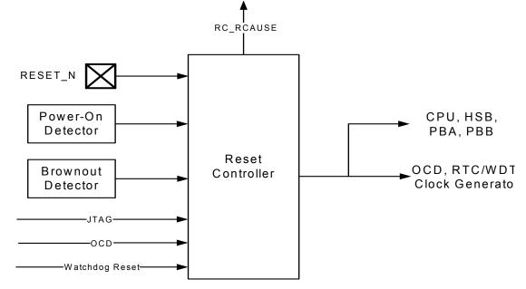
Figure 13-6. Reset Controller block diagram
