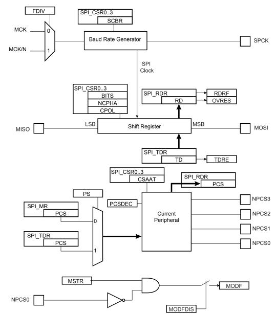
Figure 23-5. Master Mode Block Diagram
