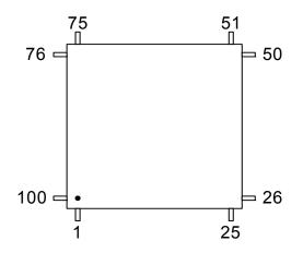
**Table 7-1.**TQFP100 Package Pinout
